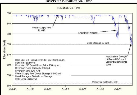
Figure 7 Reservoir Elevation vs. Time
