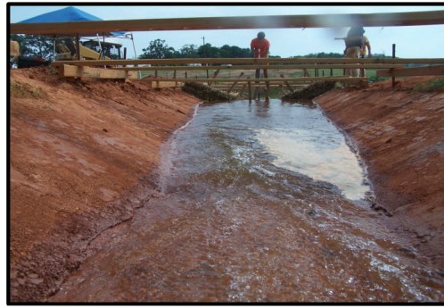
Increased Ponding and Overtopping. No Apparent Underflow
