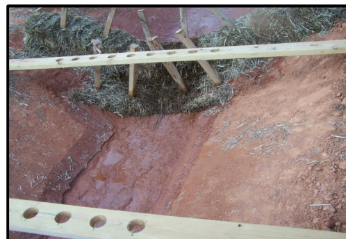
End-of-test and Post-test With Upstream Sediment Deposition and Modest Downstream Scour
