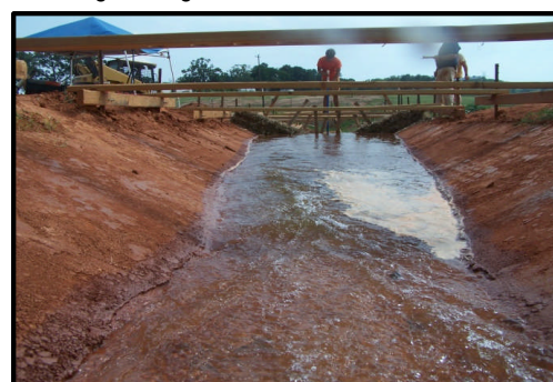
Increased Ponding and Overtopping. No Apparent Underflow
