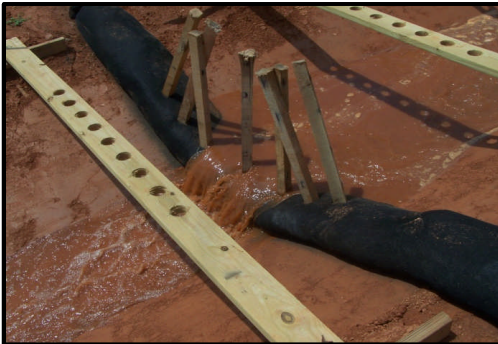
Initial Flow & Upstream Ponding with Overtopping
