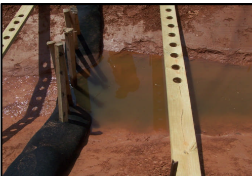
End-of-test and Post-test With Upstream Sediment Deposition
