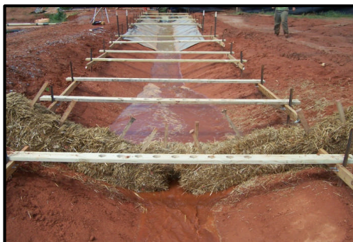
Initial Flow & Upstream Ponding with Some Underflow
