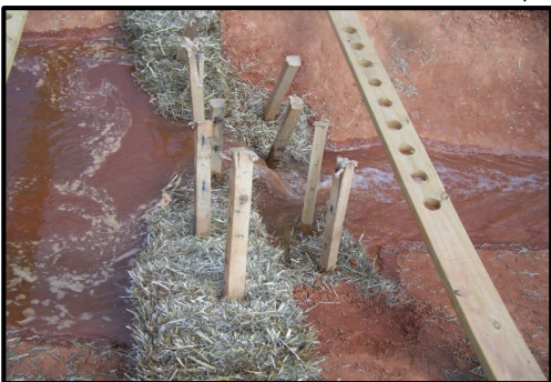
Increased Ponding and Overtopping. No Apparent Underflow
