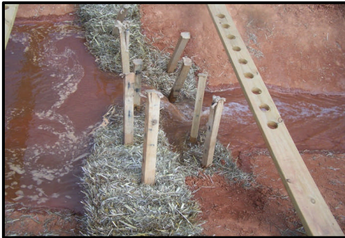
Increased Ponding and Overtopping. No Apparent Underflow
