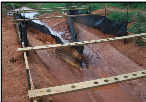
Post-test With Upstream Scour Hole
