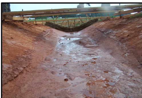
End-of-test and Post-test With Upstream Sediment Deposition and Modest Downstream Scour
