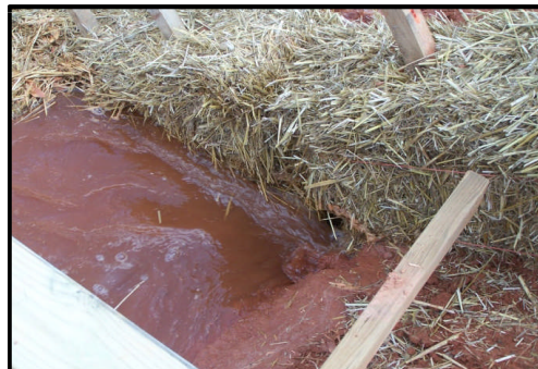
Increased Ponding, Start Overtopping, Increased Underflow
