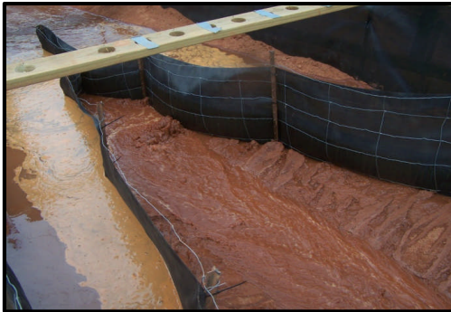
Increased Ponding Reaches Maximum and then Blows Out Under Fence
