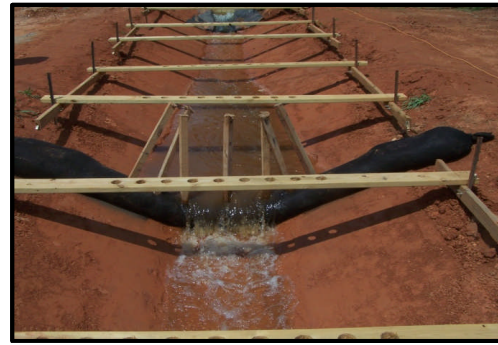
Increased Ponding and Overtopping. No Apparent Underflow
