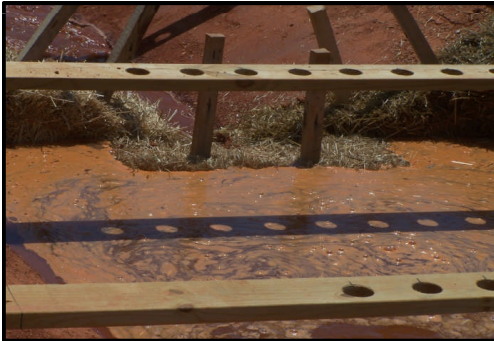
Increased Ponding and Undermining
