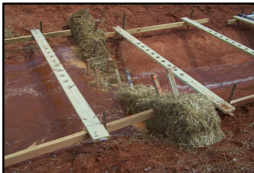
Increased Ponding, Start Overtopping, Increased Underflow
