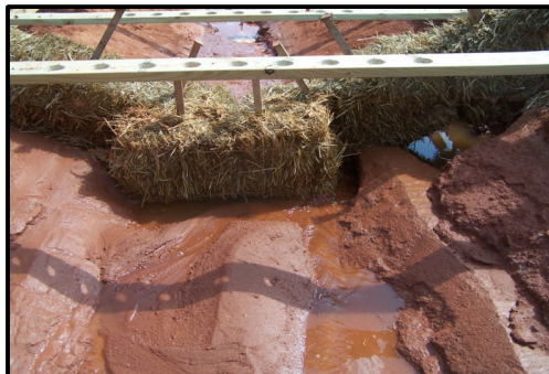
End-of-test and Post-test With Undermined Bale Removed
