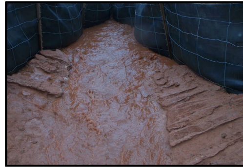
Increased Ponding Reaches Maximum and then Blows Out Under Fence
