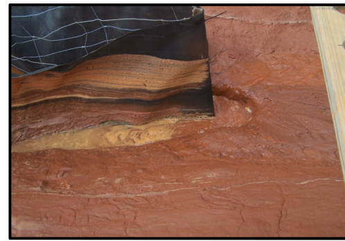
Post-test With Upstream Scour Hole
