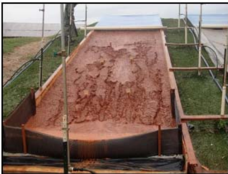
Figure 10. Type B Silt Fence End-of-Test
