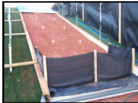
Figure 4 Typical Prepared Slope & Sediment Barrier Installation
