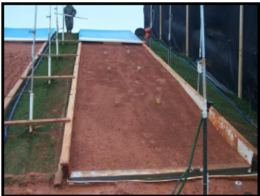
Figure 3. Typical Prepared Control Slope
