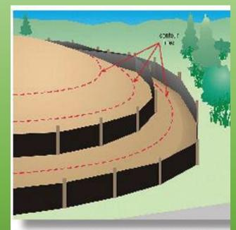
Install silt fencing on the contour, with the ends turned uphill to trap muddy runoff and prevent bypasses. Remove silt fences when grass is established.
