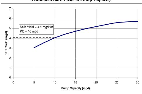
Figure 7 Estimated Safe Yield vs Pump Capacity
