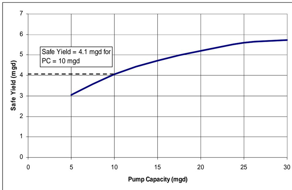
As presented in Figure 7, there is diminishing return (safe yield) with increasing pump capacity (reflecting pump station and pipeline cost). For the purposes of this analysis, an estimated economical safe yield & pump capacity combination were selected from the above graph. The
