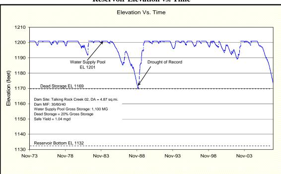
Figure 7 Reservoir Elevation vs. Time
