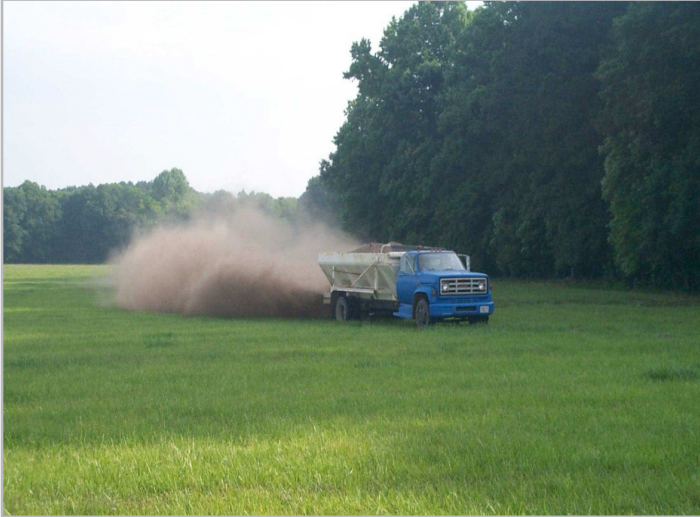
A litter spreader applies waste to a field as fertilizer
