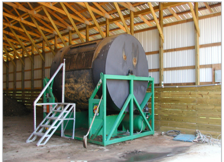
A drum composting system on a poultry farm in southwest Georgia
