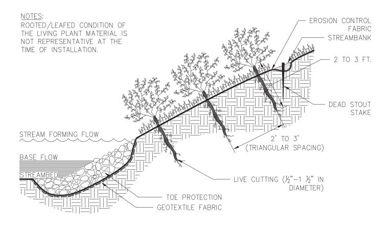
Figure 6-9.1 Illustration of a Live Stake
