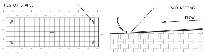
LAY NET WITH THE DIRECTION OF FLOW.
