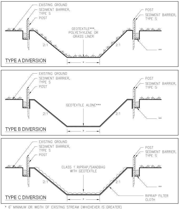
\*\* SEDIMENT BARRIER AND FILTER CLOTH SHOULD BE ENTRENCHED IN THE SAME TRENCH. \*\*\*GEOTEXTILE SHALL BE SPECIFIED IN ACCORDANCE WITH AASHTO M288–96 SECTION 7.5
