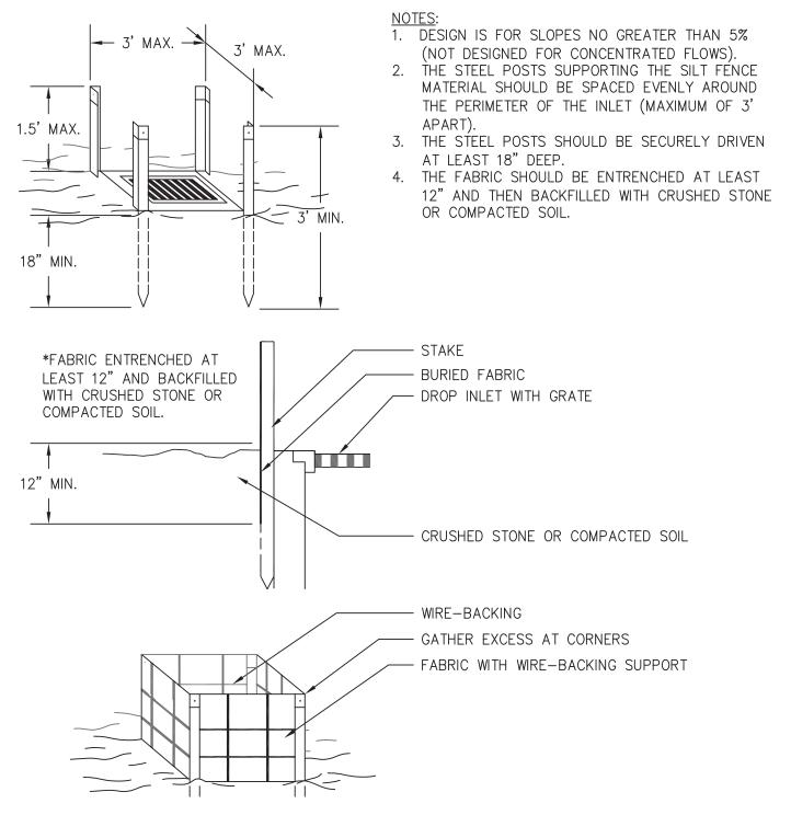
Figure 6-28.1 - Fabric and Supporting Frame For Inlet Projection
