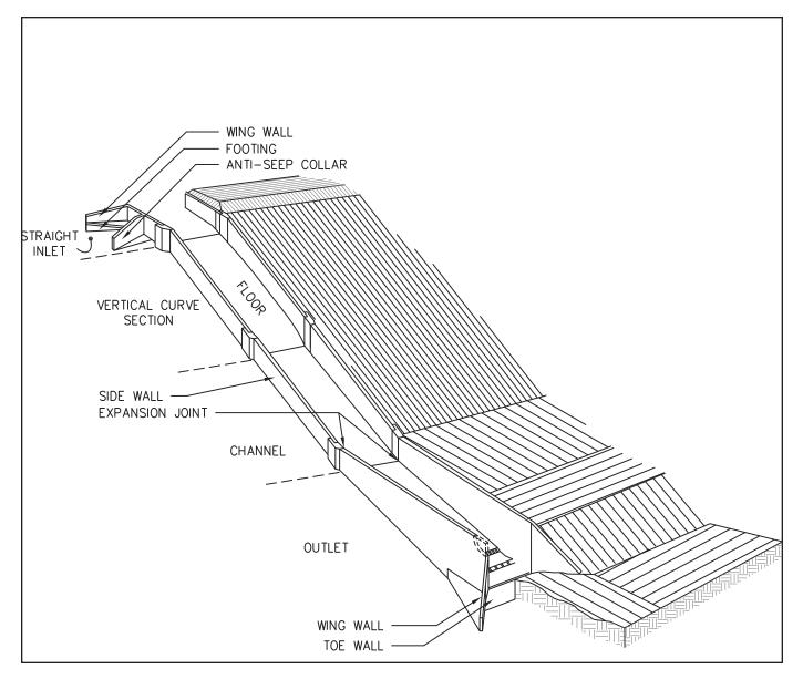
Figure 6-22.7 Chute Spillway
