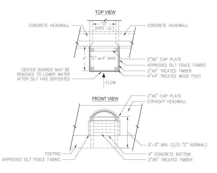
Figure 6-26.3 Slotted Board Dam with Stone or Filter Fabric
