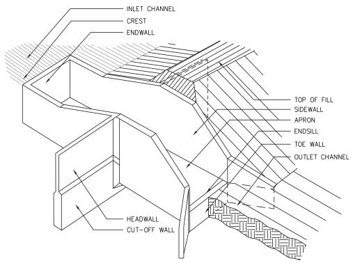
Figure 6-22.6 Box Drop Inlet Spillway
