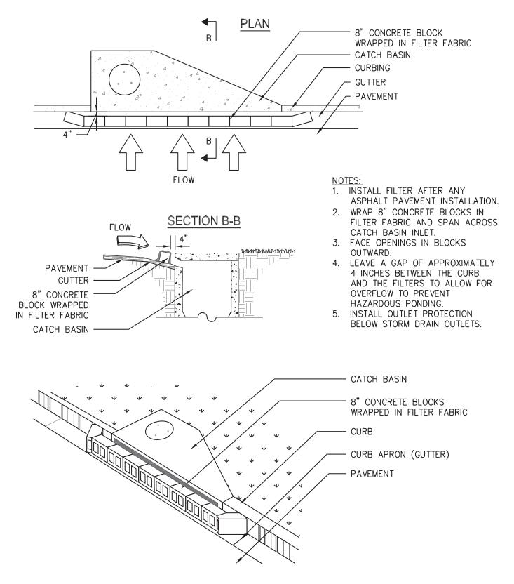
Figure 6-28.6 Curb Inlet Filter "Pigs in Blanket"
