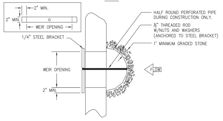
Figure 6-26.1 Perforated Half- Round Pipe with Stone Filter
