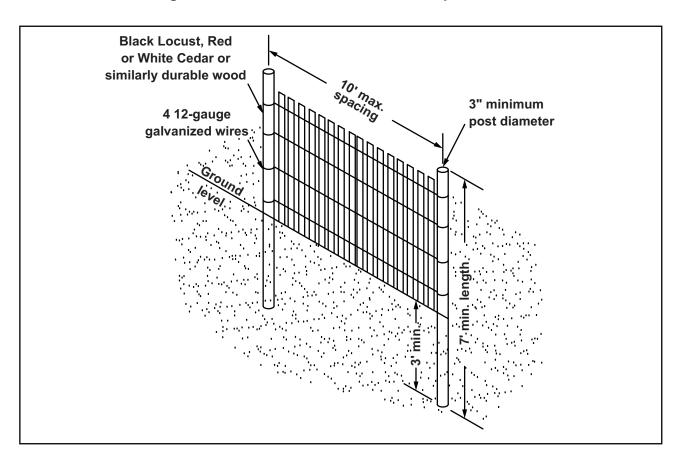
Figure 6-2.2 - Sand Fence Installation Requirements
