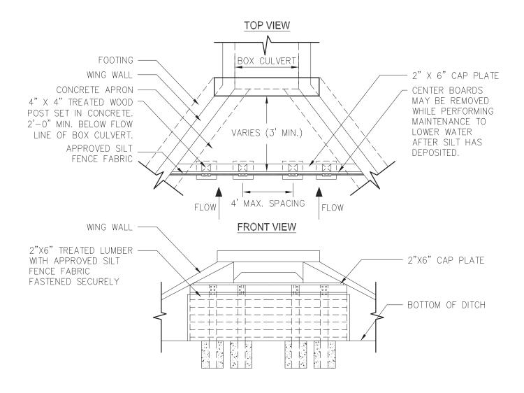
Figure 6-26.4 Silt Control Gate
