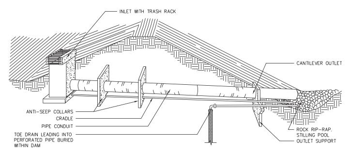
Figure 6-22.5 Drop Inlet Spillway
