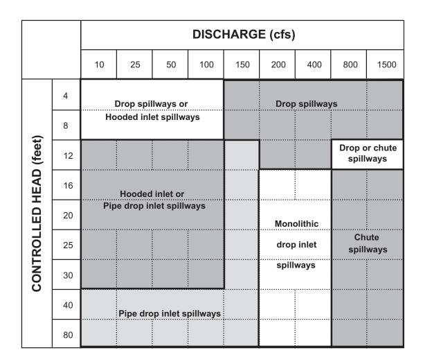
Note: Chart shows most economical structure as related to discharge and controlled head providing site conditions are adequate.
