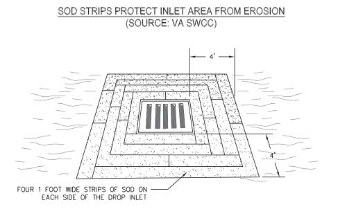
Figure 6-28.5 Sod Inlet Protection
