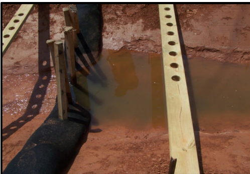
End-of-test and Post-test With Upstream Sediment Deposition
