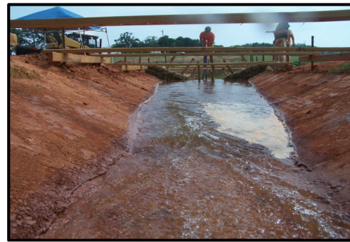
Increased Ponding and Overtopping. No Apparent Underflow
