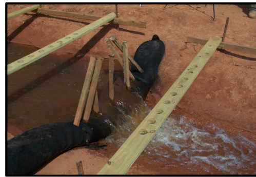
Increased Ponding and Overtopping
