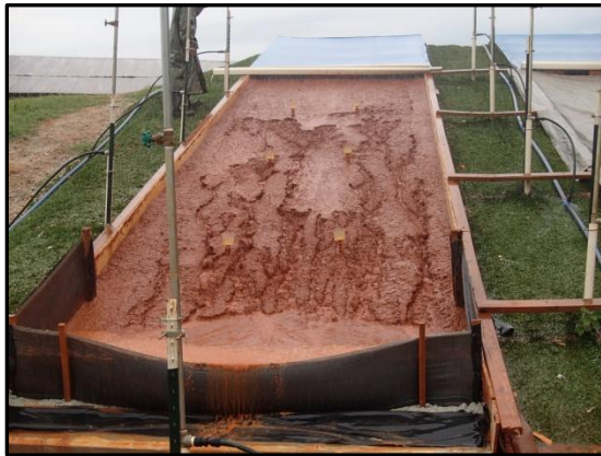
Figure 10. Type B Silt Fence End-of-Test
