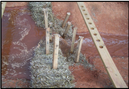
Increased Ponding and Overtopping. No Apparent Underflow
