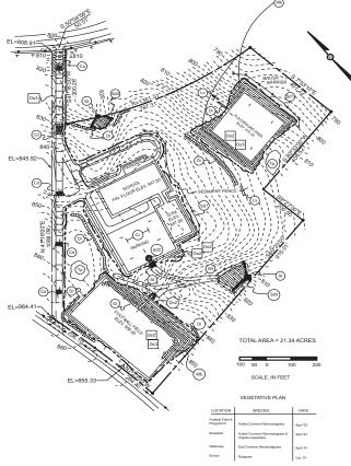
Figure 2.3 - Permanent facilities for this development were planned to fit the topography and soil type.
