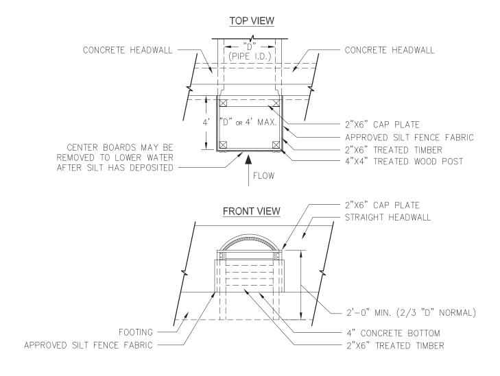
Figure 6-26.3 Slotted Board Dam with Stone or Filter Fabric
