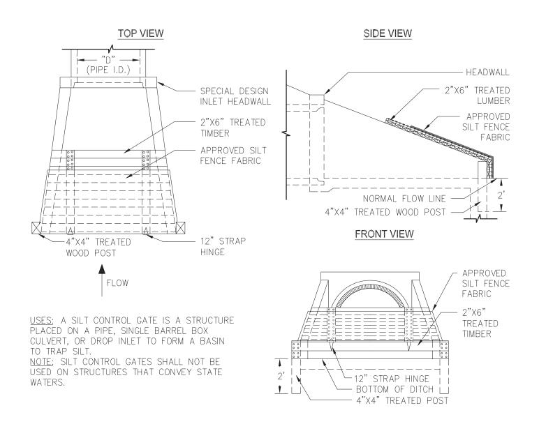
Figure 6-26.5 Silt Control Gate
