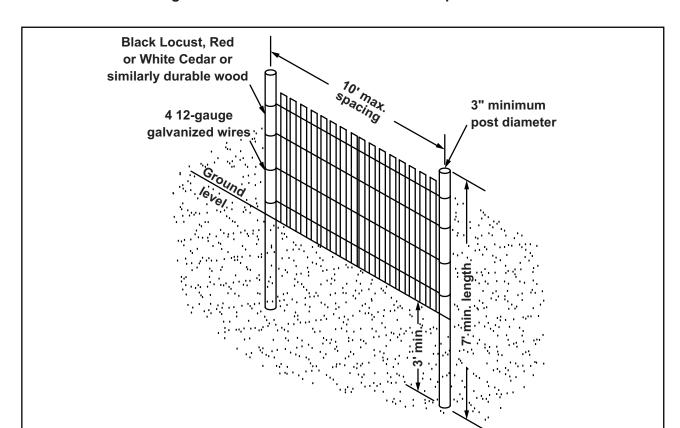
Figure 6-2.2 - Sand Fence Installation Requirements
