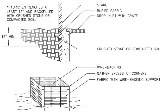
Figure 6-28.1 - Fabric and Supporting Frame For Inlet Projection
