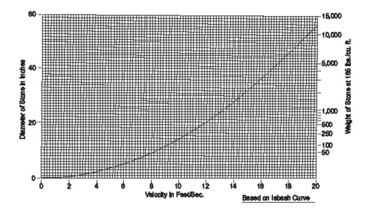
Figure C-1. - Maximum Stone Size for Riprap
