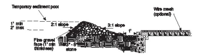
Figure 6-28.4 Gravel Drop Inlet Protection
