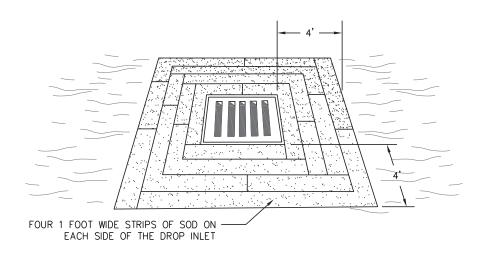
Figure 6-28.5 Sod Inlet Protection
