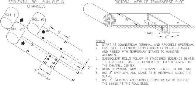
Figure 6-10.1 - Typical Installation Guidelines for Matting and Blankets
