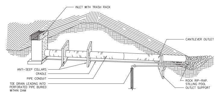
Figure 6-22.5 Drop Inlet Spillway
