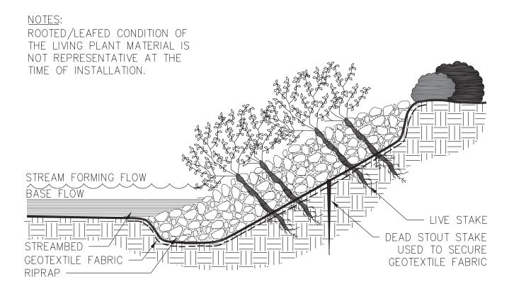
Figure 6-9.5 Illustration of Joint Planting
