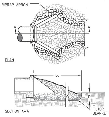
Figure 6-34.3 - Riprap Outlet Protection (Modified From Va SWCC)
