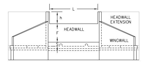
Figure 6-22.3 - Symbols For Straight Drop Spillway
