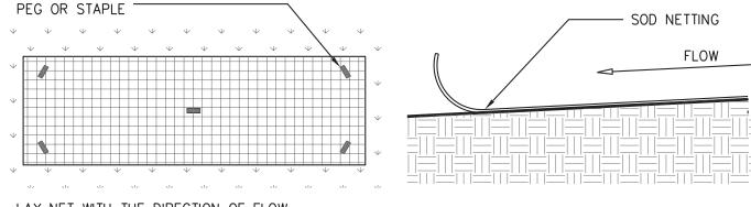
LAY NET WITH THE DIRECTION OF FLOW.
