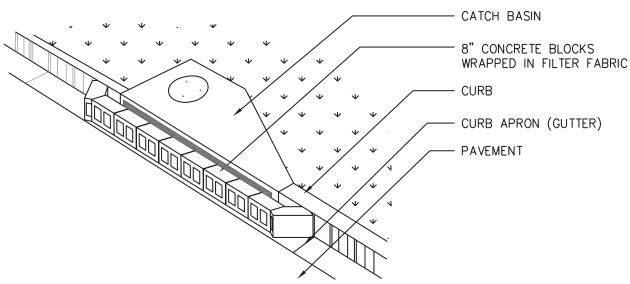
Figure 6-28.6 Curb Inlet Filter "Pigs in Blanket"
