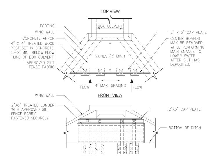
Figure 6-26.4 Silt Control Gate
