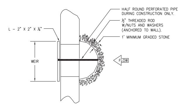
Figure 6-26.1 Perforated Half- Round Pipe with Stone Filter
