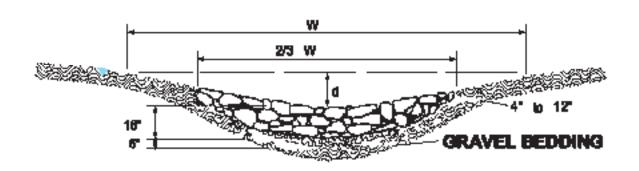
Waterway with stone center drain Rounded section shaped by buildozer
