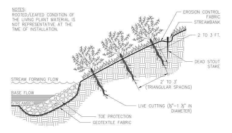
Figure 6-9.1 Illustration of a Live Stake
