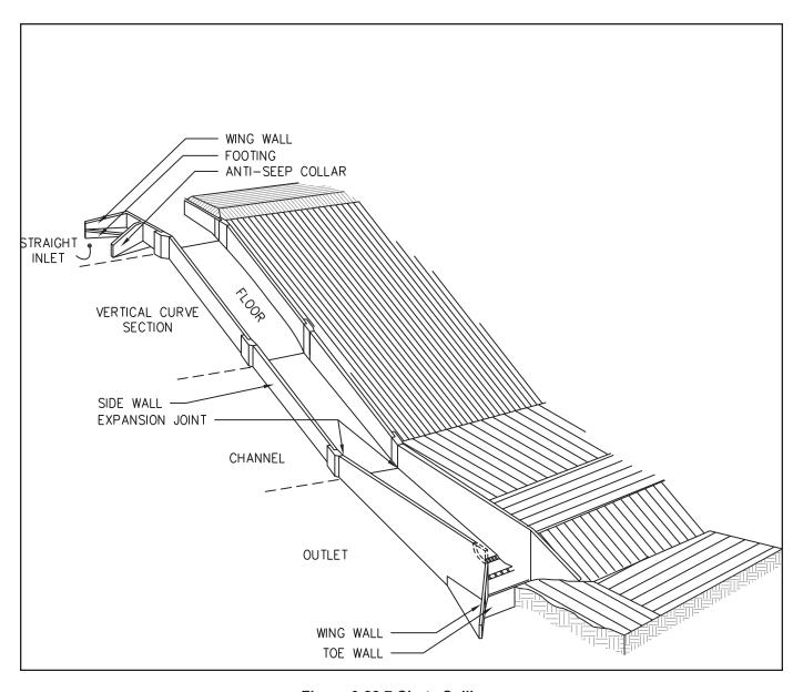
Figure 6-22.7 Chute Spillway
