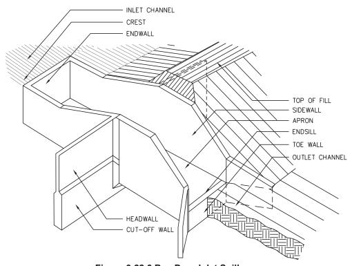
Figure 6-22.6 Box Drop Inlet Spillway
