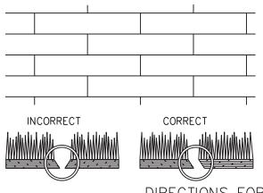
LAY SOD IN A STAGGERED PATTERN. BUTT THE STRIPS TIGHTLY AGAINST EACH OTHER. DO NOT LEAVE SPACES AND DO NOT OVERLAP. A SHARPENED MASON'S TROWEL IS A HANDY TOOL FOR TUCKING DOWN THE ENDS AND TRIMMING PIECES.
